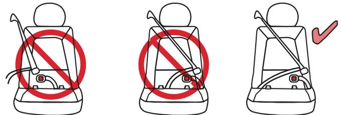
The vehicle belt fits properly when the lap part sits low across the child's upper thighs (b) and the shoulder part lies across the center of the child's chest and does not contact the child's neck when routed through the upper belt guide (a).
