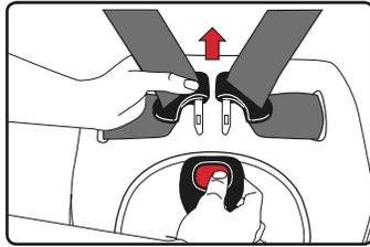
Press the release button and pull the tongues from the buckle.
