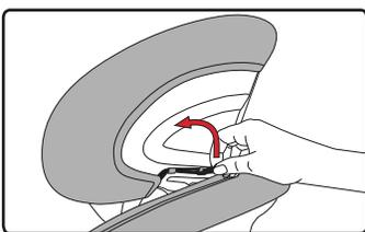
**6** Unhook the elastic bands, then remove the side wing covers from each side of the child seat shell.
