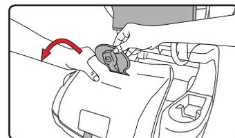
**7 Turn and pull the buckle retainer through the slot in the child seat shell.**
