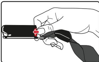
2 Pull the lower connector from the storage slot or lower anchor.
