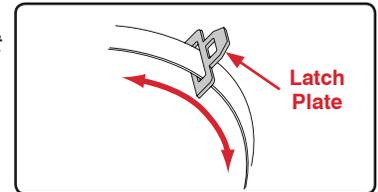
**b** Has a retractor that can be switched to function as an ALR by pulling the vehicle belt fully out until a clicking sound can be heard when retracting.
