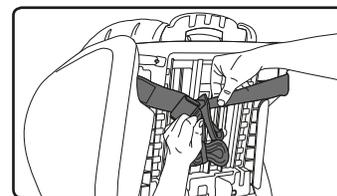
2 Firmly press the hook over the a tether anchor point.
