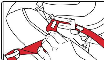
**TIP:** Raising the head restraint to the highest position will allow for easier access to the shoulder belt guide.
