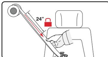
**c** Tightens by feeding the belt webbing back into the retractor.
