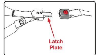
**NOTE:** To use a child seat with this type of vehicle belt, you will need to switch the retractor for the lap section of the seat belt to the ALR mode.
