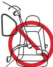
Lap-shoulder belts with top or bottom anchor points on the vehicle door.
