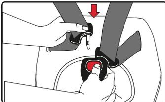
**9 Pull the adjuster strap to tighten the harness.**
