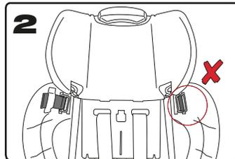
**IMPORTANT:** Discontinue use of child seat if it has been involved in a moderate or severe crash, regardless of whether the loops have pulled through the back side of the shell and the colored stitching has been ripped.
