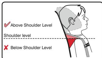
**IMPORTANT:** In booster mode the vehicle belt must be in the closest position at or above the child's shoulder through the shoulder belt guide.
