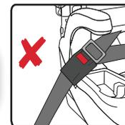
If the buckle lies near the incorrect position (X) when the vehicle belt is tightened, try fitting the child seat in another seating position in the vehicle. If it is not possible to achieve the correct position (✓) for the buckle, then another seating position **MUST** be used.
