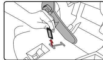
**Booster to Harness Mode: Replacing the Harness and Buckle**
