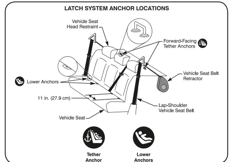
The Lower Anchors and Tethers for Children or LATCH, is a system available on this child seat that offers an alternative to vehicle seat belt installation methods. The figure above shows typical locations for lower anchors and tether anchors in a vehicle. See pages 2-3 for LATCH components on this child seat.
