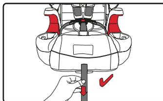
**Harness to Booster Mode: Removing the Harness and Buckle****1 Loosen the harness completely.**
