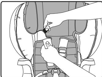
**4** Unhook the top elastic bands on each side of the head restraint.
