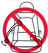
Lap belts with a sewn-in latch plate that have a retractor that locks only in case of a sudden stop.
