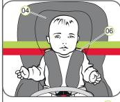
A correctly adjusted headrest 04 ensures optimal protection for your child in the safety seat: The headrest 04 must be adjusted so that the shoulder straps 06 are at the same level as your child's
