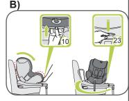
The DUALFIX has a grey safety button 20 which must be pressed when changing between group 0+ and group 1. The grey safety button 20 prevents that the child seat is used by mistake in the wrong group for your child.
